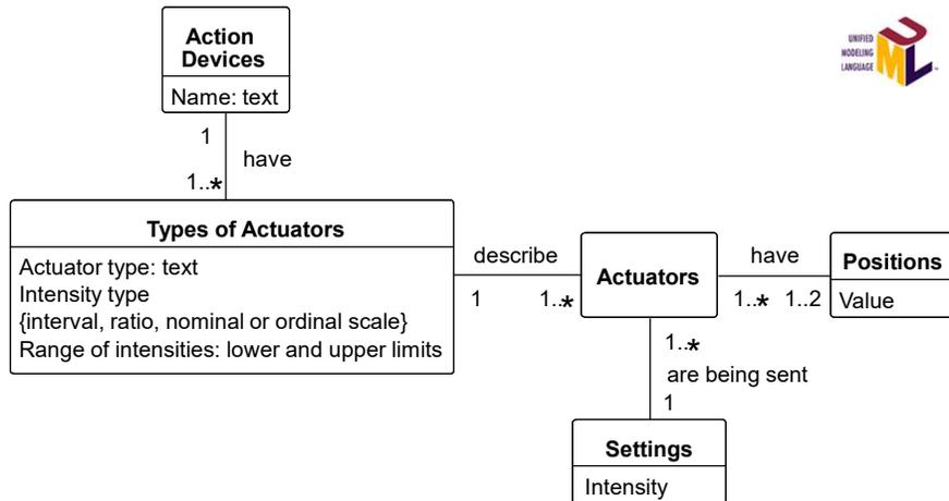
This a UML class diagram for action devices and actuators.
