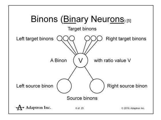
A binon is a neural node in a network [5]. It has two source nodes but connects with multiple target nodes. Source binons are closer to sensors and motor/action devices. So they are more general. Source binons represent the more primitive properties, features and actions. They are reused by multiple target binons.
