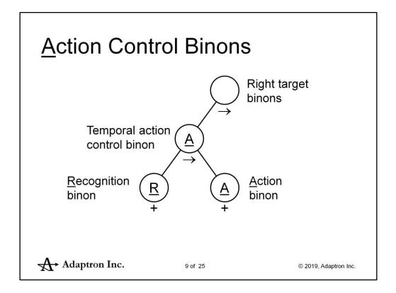
There are two types of temporal control binon: the action control and expectation control binon. The underlined letters in the binons ( $\underline{R}$ ,  $\underline{A}$  and  $\underline{E}$ ) indicate the role they play in the process. The process is equivalent to the If recognize a percept then do an action production rule.
