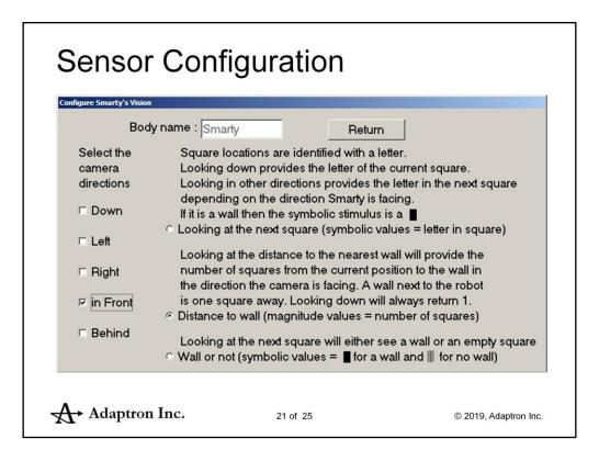
The robot body can be configured with sensors and action devices (wheels) as shown. Sensors are cameras and a motion detector. Cameras can be configured to see a letter in a square, the distance to a block (non-symbolic stimulus) or an adjacent block or empty square.
