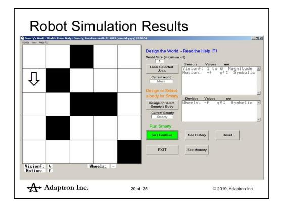
The perception-action hierarchy implemented using action and expectation binons has been successfully implemented in a simulated robot called "Smarty". It explores any designed maze world given a configuration of sensors and wheels. As illustrated, the simulation allows for a world to be designed on a grid of squares up to 8x8 in size. Each square is represented by a letter of the alphabet for symbolic stimulus recognition.
